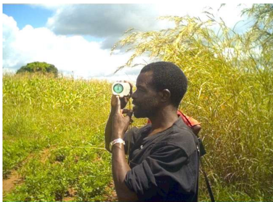
Figure 18. Mr. Phiri is measuring the slope angle.
